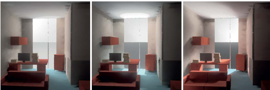
Simulated daylighting distribution in an office room through a Laser Cut Panel (LCP) at noon, 3PM and 5PM on Spring equinox.
