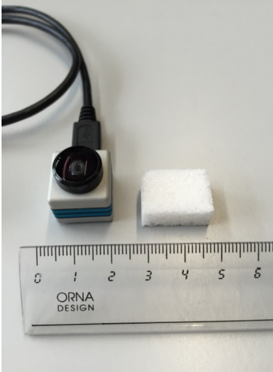
Latest HDR vision sensor Vision-In-Package (VIP) issued from CSEM
