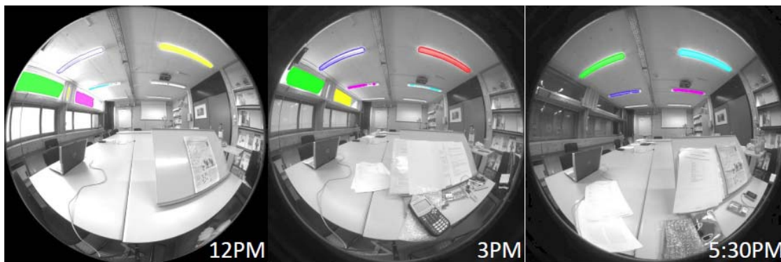
Glare sources are indicated with different colors and quantified using 'Evalglare' (Wienold & Christoffersen, 2006).
